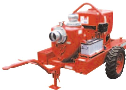
Emergency pump with silenced diesel engine
